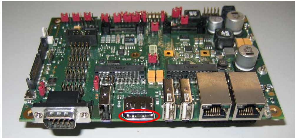
Figure 3 Connection of DisplayPort Monitor Cable
