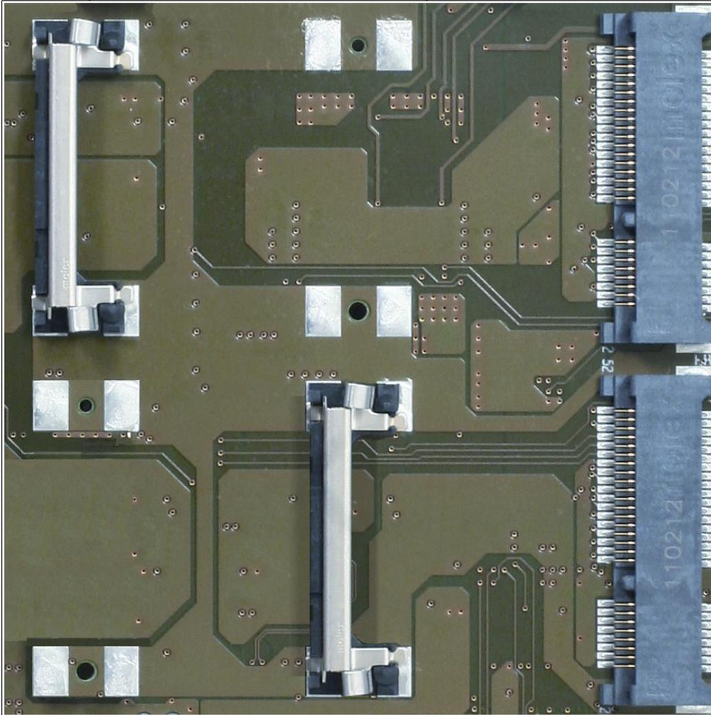
The different card sized can be easily handled on the Carrier Board by having the latches optionally placed on the full size position or on the half size position as shown in Figure 13 above.
