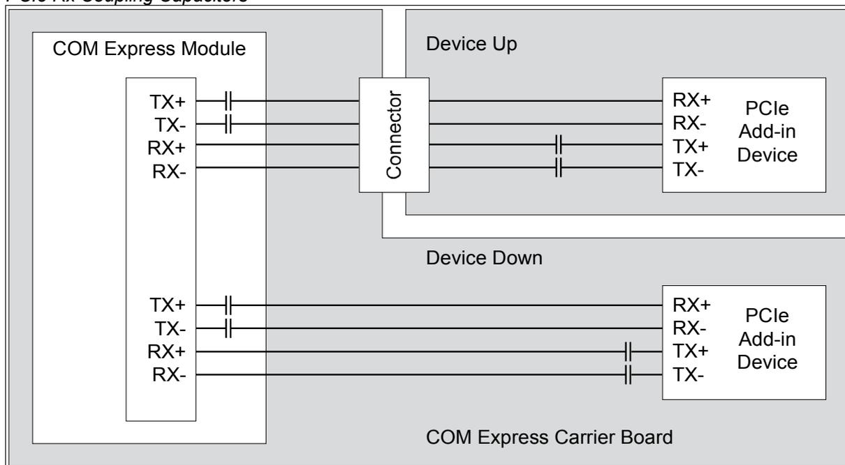
“Device Down” refers to a PCIe target device implemented down on the Carrier Board. “Device Up” refers to a PCIe target device implemented on a slot card (or mini-PCIe card, ExpressCard, AMC card). There are several distinctions between a PCIe “Device Down” and “Device Up” implementation:
