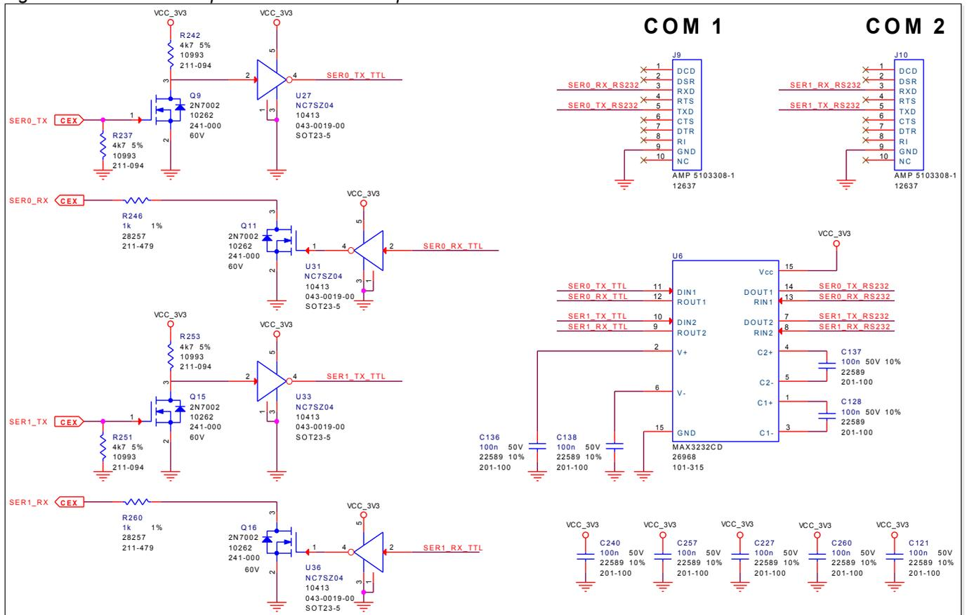
Figure 49: General Purpose Serial Port Example shows the schematic of two general purpose serial ports with RS232 level shifter (U6). The transistor / inverter combination at the serial TX and RX lines coming from the Module is necessary to handle the protection against VCC\_12V connection according to chapter 5.10 of COM.0 Rev. 2.1. The MAX3232CD is a dual port RS232 transceiver and handles the level shifting of the TTL signals to the regarding voltage level.
