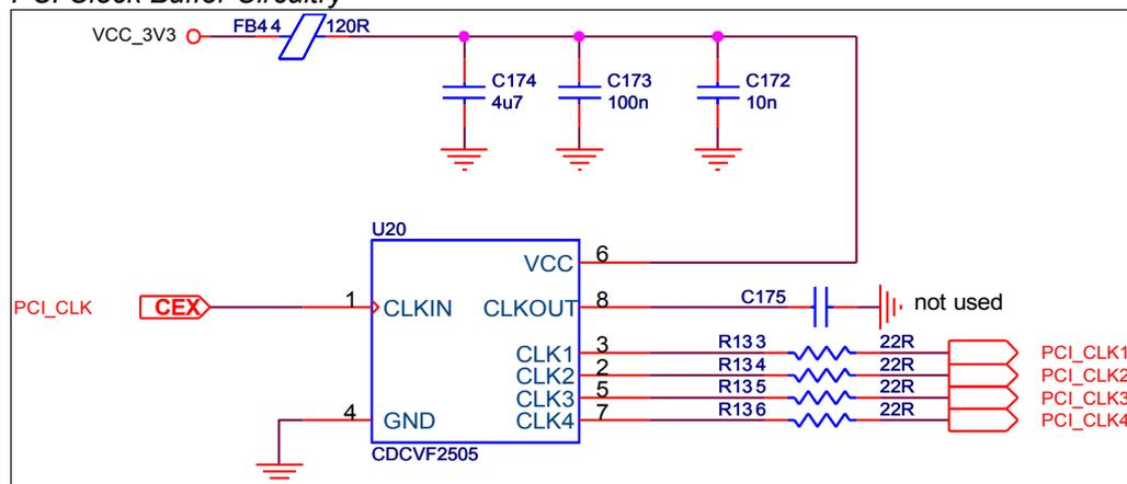
**Note:** *In accordance with the 'PCI Local Bus Specification Revision 2.3', the PCI clock signal requires a rise and fall time (slew rate) within 1V/ns and 4V/ns. The slew rate must be met across the minimum peak-to-peak portion of the clock wave form, which is between 0.66V and 1.98V for 3.3V clock signaling. These parameters are very critical for EMI and must be observed during Carrier Board layout when implementing the PCI Bus.*
