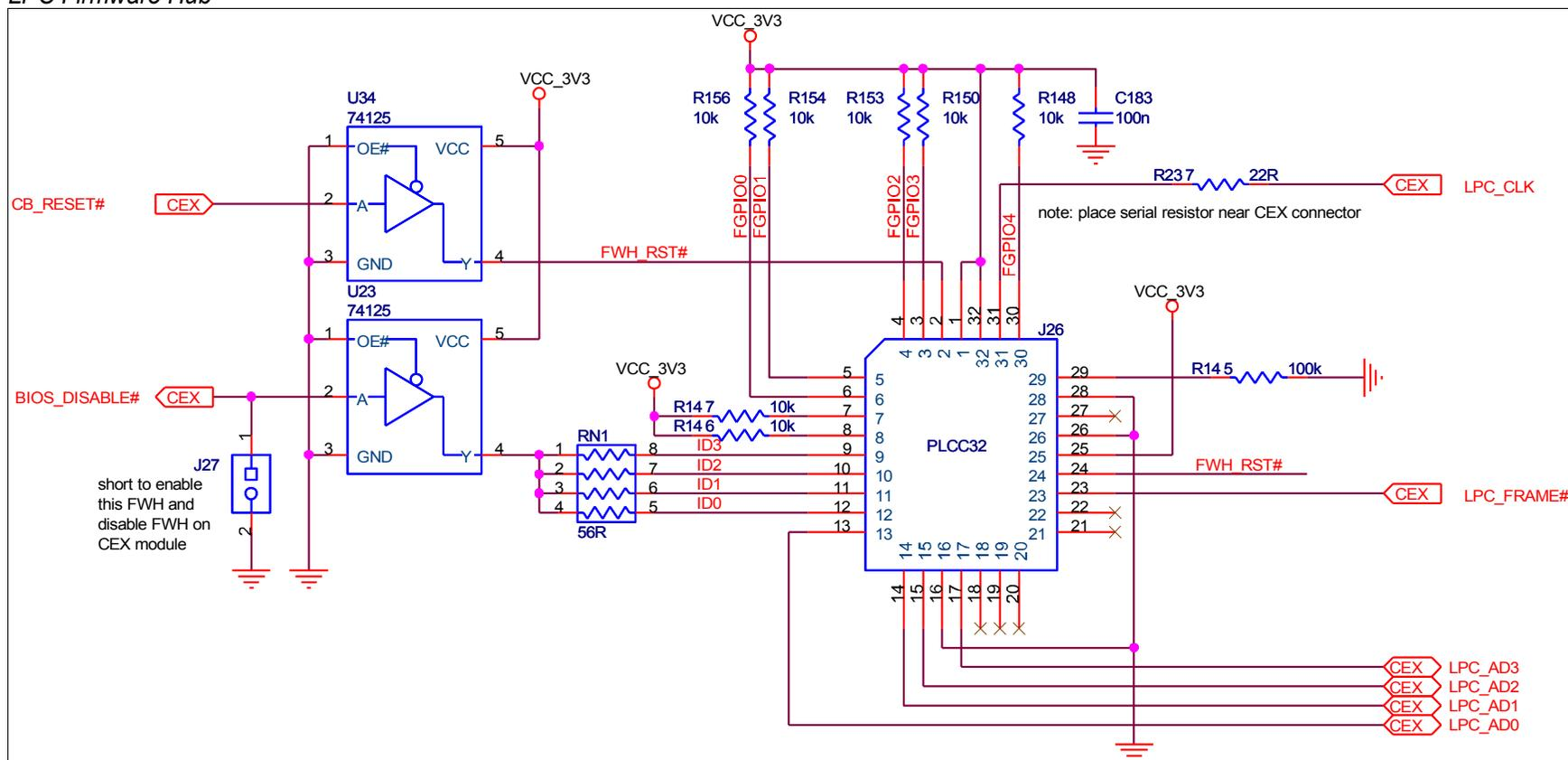
The BIOS device shown in Figure 80: LPC Firmware Hub above is a SST SST49LF008A Firmware Hub in a 32-pin PLCC package. The socket used is a 32-pin PLCC socket, AMP/Tyco 822498-1. This is a surface-mount socket, and PCBs can be laid out such that the socket or the FWH itself is soldered to the Carrier Board.
