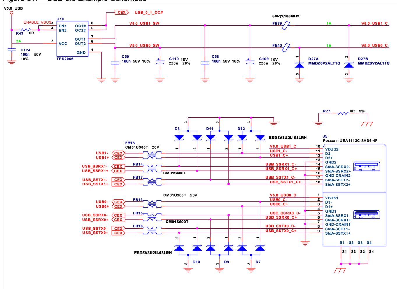
J5 incorporates a dual USB 3.0 Type A host receptacle. Note that the SuperSpeed pins are separate from the USB 2.0 pins.
