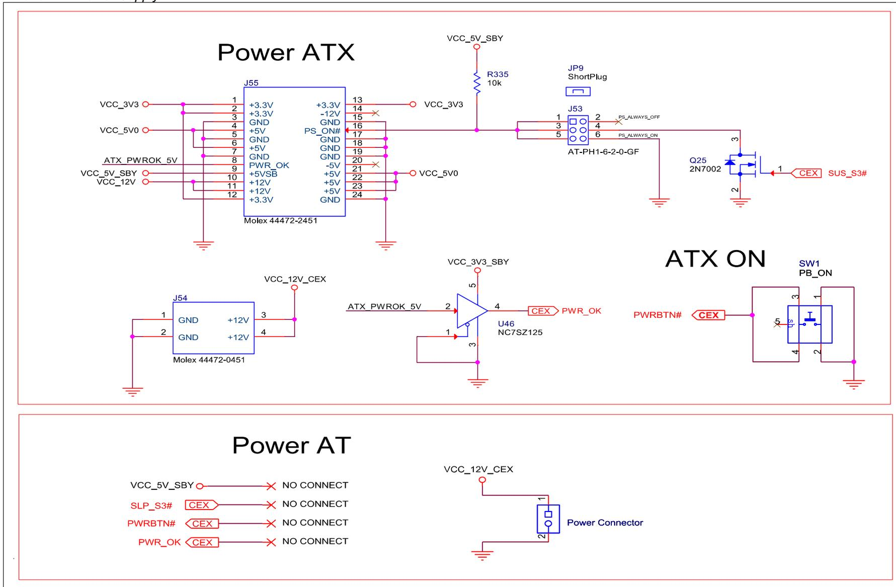
The PWRBTN# signal is an input to the COM Express Module. Switch de-bouncing is done on the Module. The falling edge of the PWRBTN# signal can initiate a state transition from S5 (soft off) to S0 (full on). It may also cause the reverse transition, to S5, if the unit is in one of the 'on' states.
