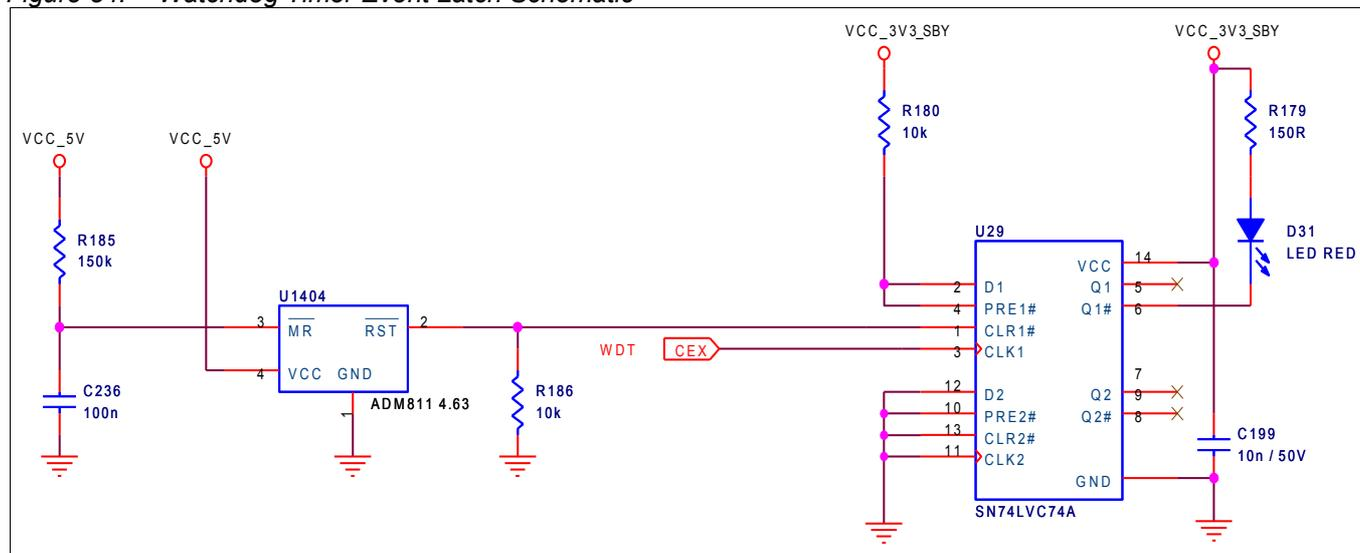
The Watchdog Timer (WDT) event signal is provided by the COM Express Module. The WDT output is active-high. It is sourced from Module pin B27.
