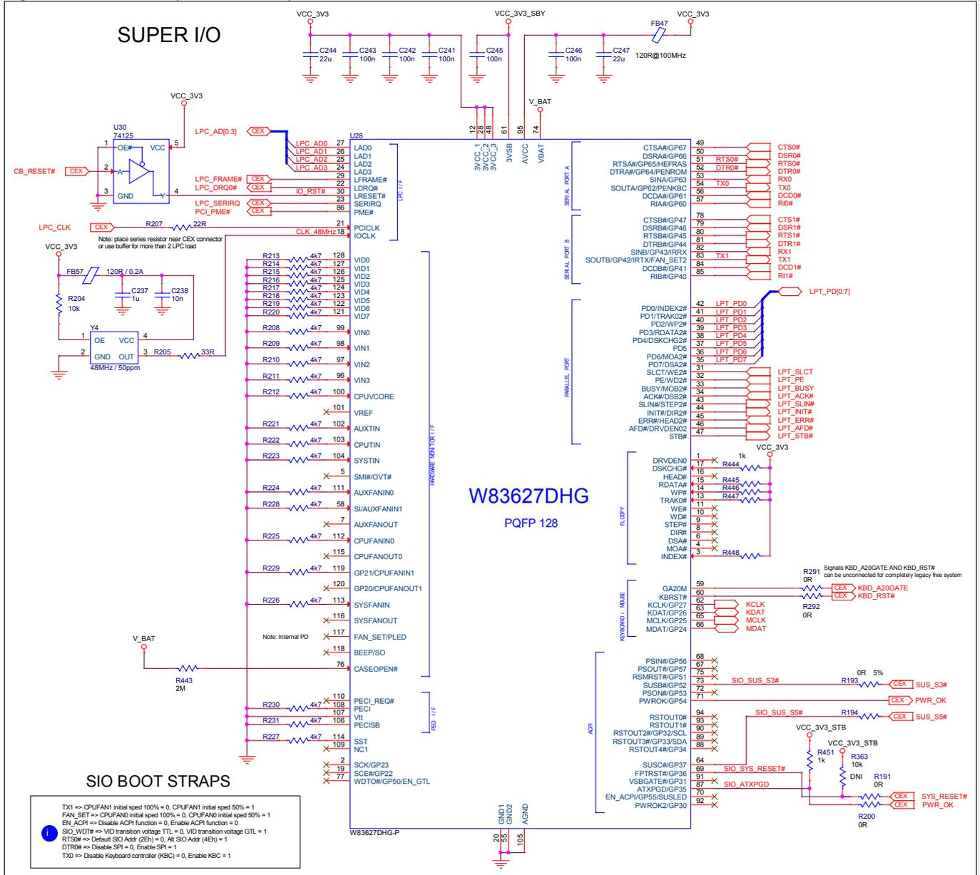
Figure 45: LPC Serial Interfaces
