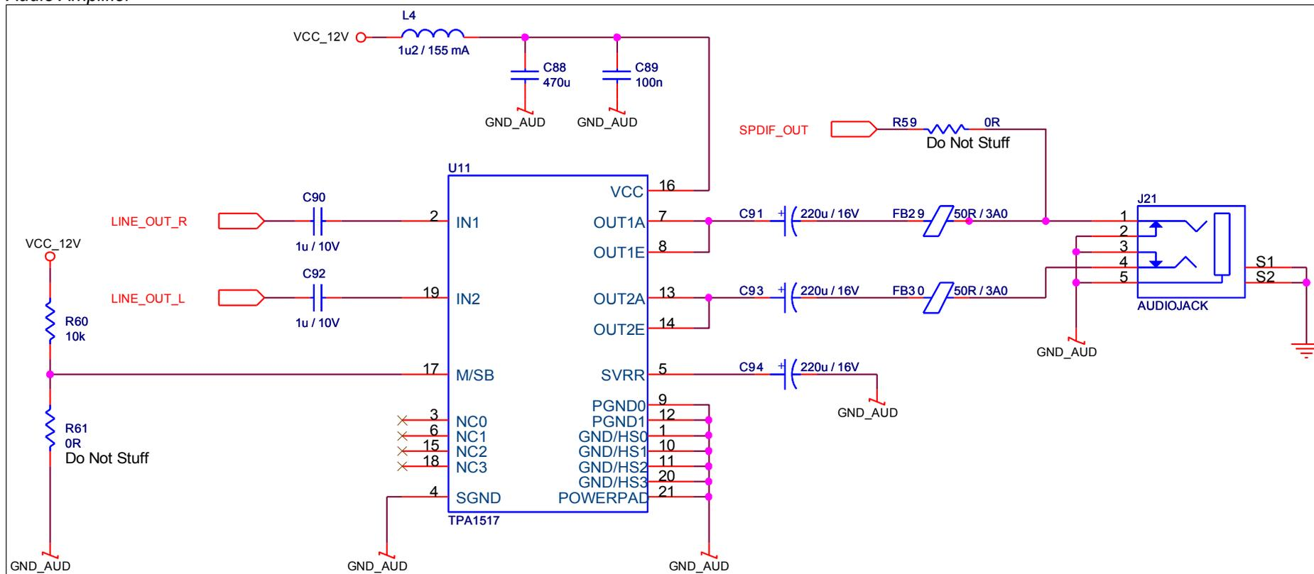
The example above shows a traditional class AB amplifier. There are many physically smaller and more power efficient class D audio amplifier options from vendors such as Texas Instruments, NXP and others.
