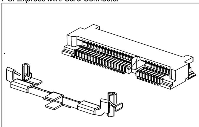
A typical PCI Express Mini-Card socket is shown in Figure 12 above.
