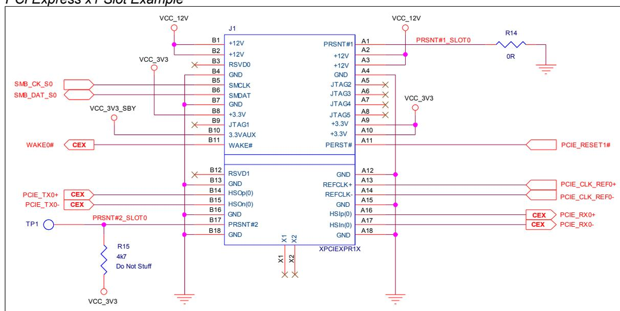
The example above shows COM Express PCIe lane 0 connected to the slot. Other lanes may be used, depending on what is available on the particular Module being used.
