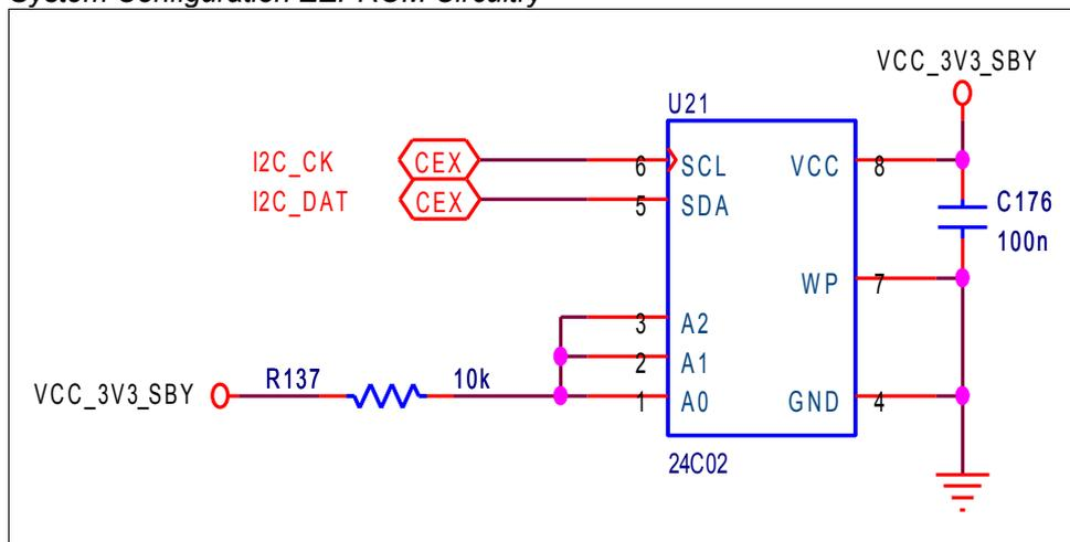
The EEPROM stores configuration information for the system of the Carrier Board. The data structure used is defined in the PICMG EEPROM Specification. The Specification recommends but does not require the use of this system configuration EEPROM. The Module BIOS may check the Carrier Board configuration EEPROM but is not required to do so by the Specification.
