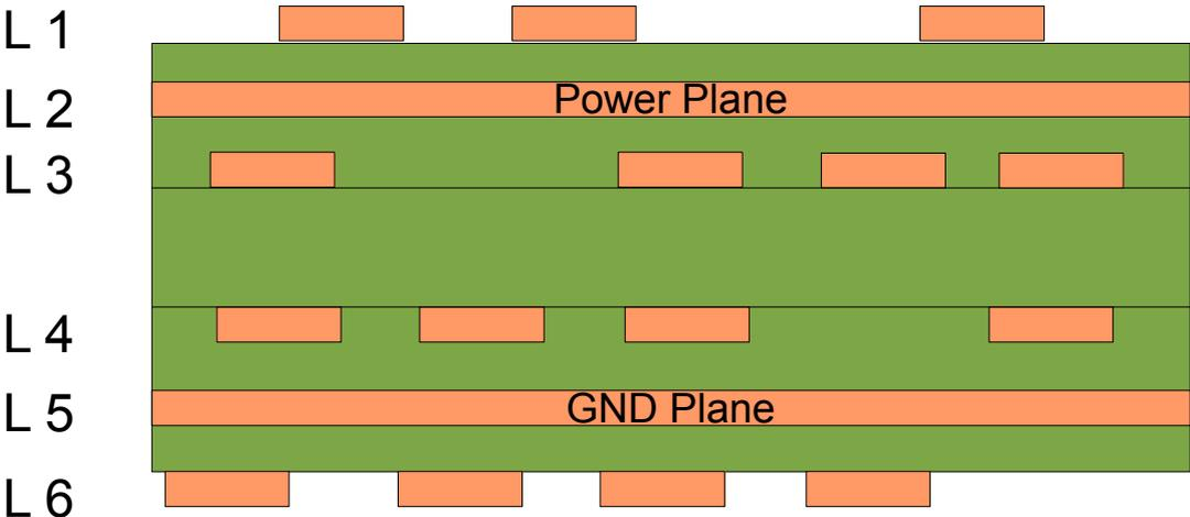
Figure 69 above is an example of a six layer stack-up. Layers L1, L3, L4 and L6 are used for signal-routing. Layers L2 and L5 are power and ground planes respectively.
