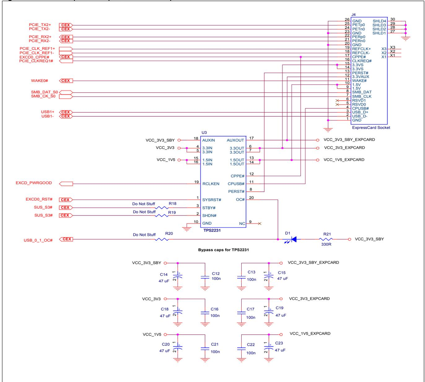
Figure 17 above shows an ExpressCard implementation. The example shows COM Express PCIe lane 2 and USB port 1 used, but other assignments may be made depending on Module capabilities and the system configuration.
