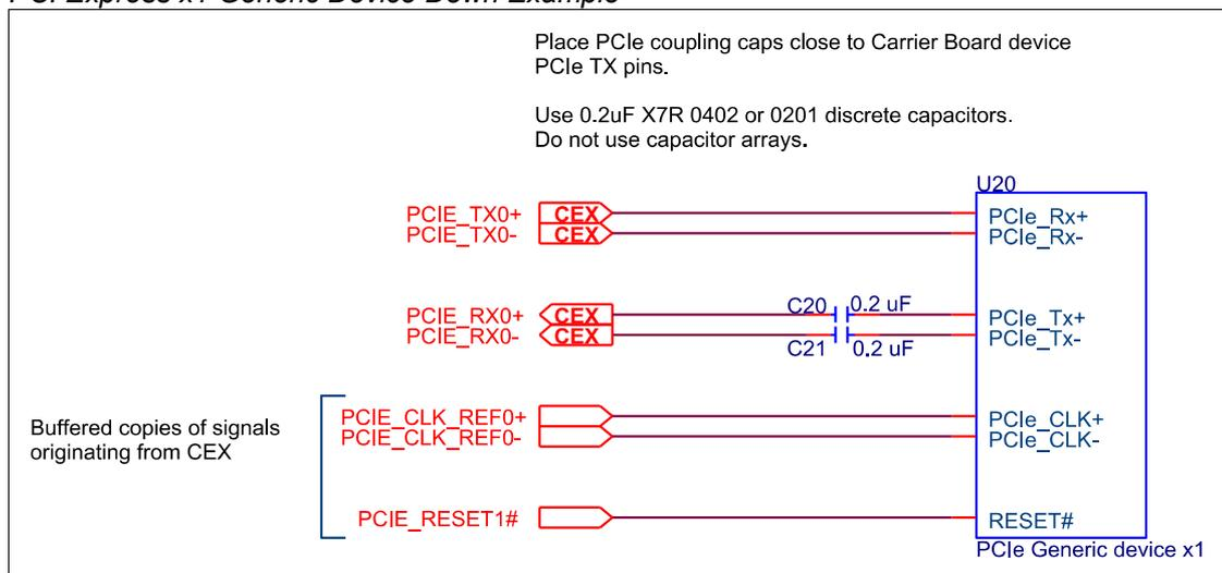
A generic example of a PCIe x1 device on a COM Express Carrier Board is shown in the figure above. Only the signals that interface to the COM Express Module in the full power-on state (S0) are shown here.
