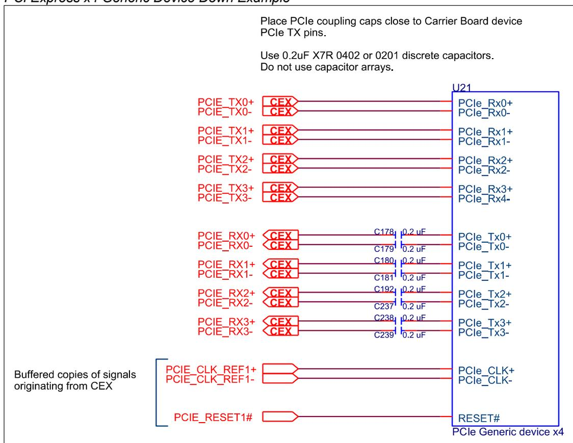
A generic example of a PCIe x4 device on a COM Express Carrier Board is shown in the figure above. Only the signals that interface to the COM Express Module in the full power-on state (S0) are shown here.
