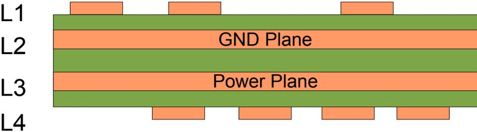
Figure 68 above is an example of a four layer stack-up. Layers L1 and L4 are used for signal routing.
