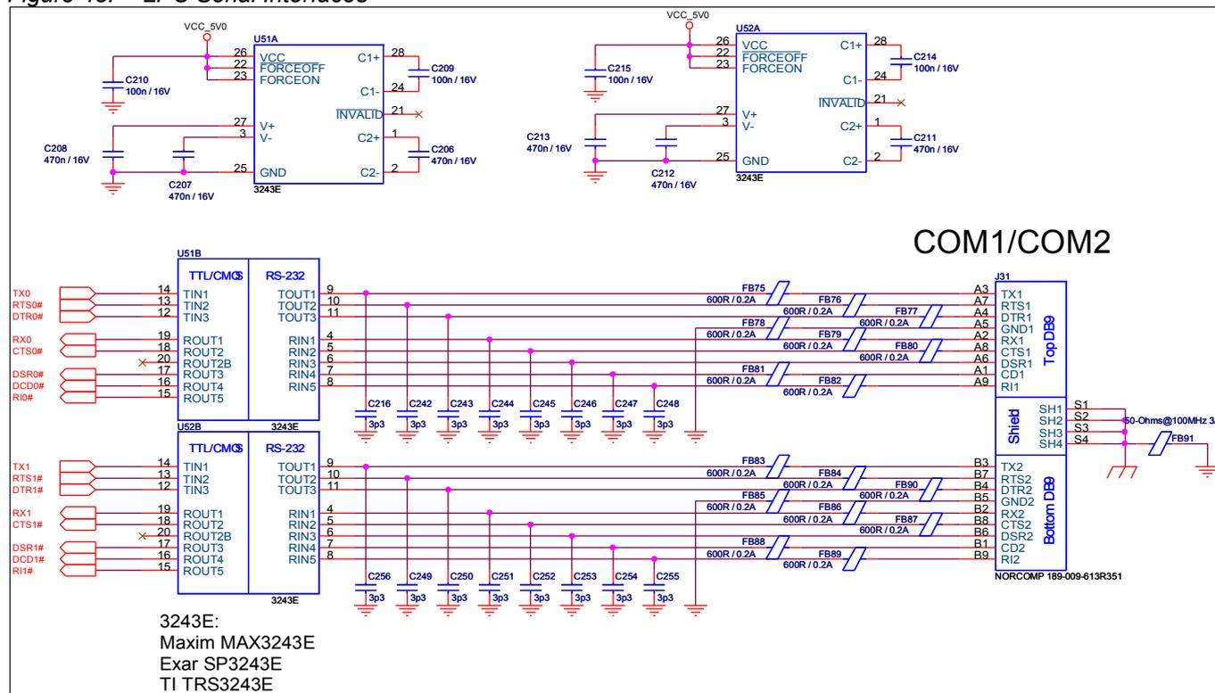
**Note:** Connection between logic GND and chassis depends on grounding architecture. Connect GND with chassis at a single point even though this connection is drawn on all schematic examples throughout this document.
