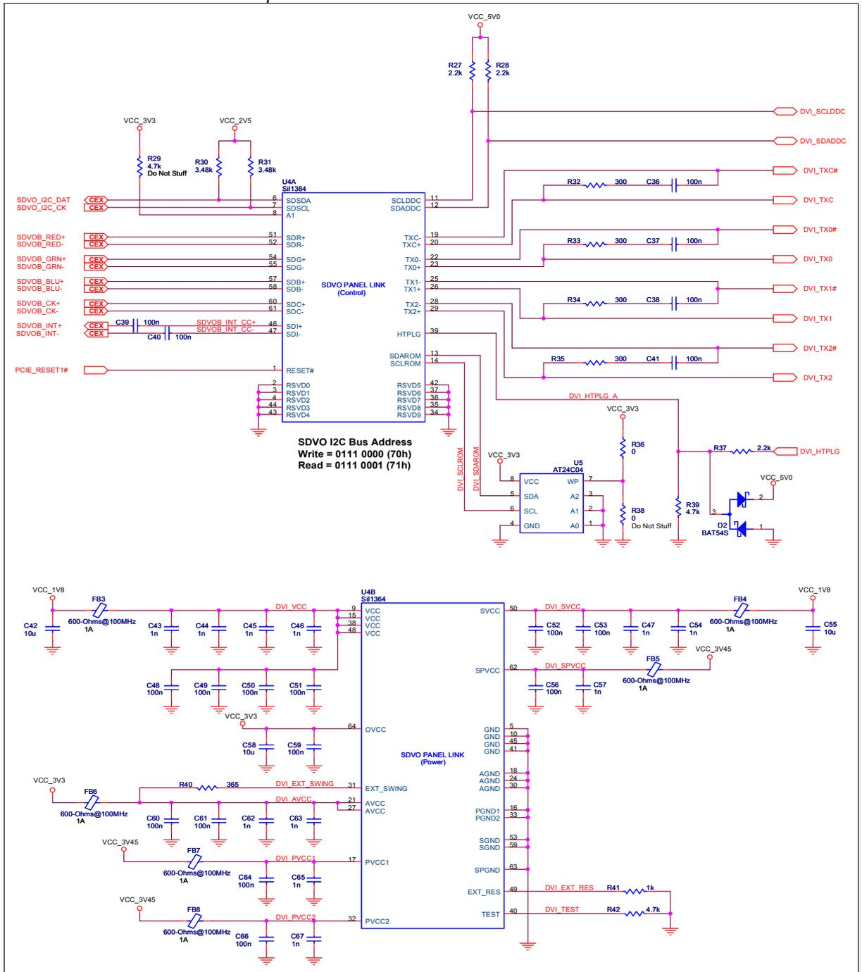
Figure 23 'SDVO to DVI Transmitter Example' above shows a single-channel, device-down application for SDVO to DVI implementation. A Silicon Image transmitter IC (SIL1364) converts SDVO signals from the Module to a DVI-D format. Pins are connected to the DVI-D Connector (Molex 74320-4004).
