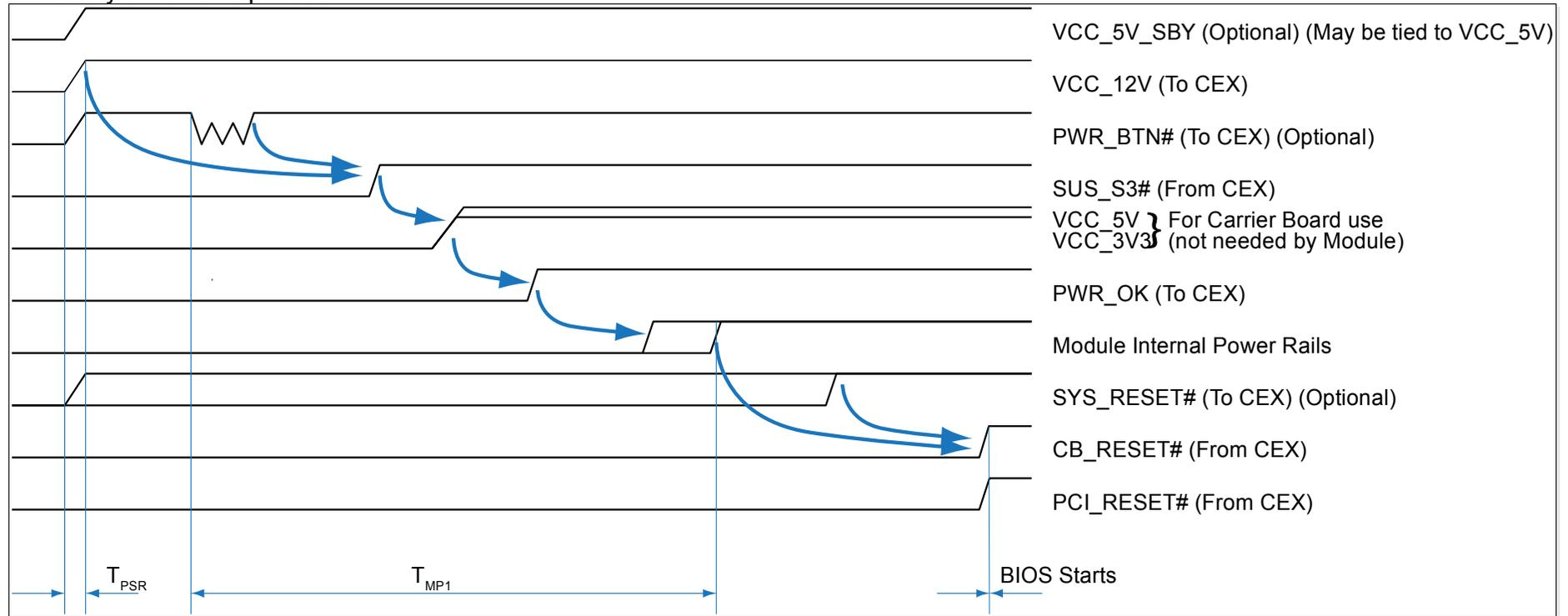
Table 53 below indicates roughly what time ranges can be expected during the boot process, per Figure 64 and 65 above. Check with your Module vendor if more specific information is required.
