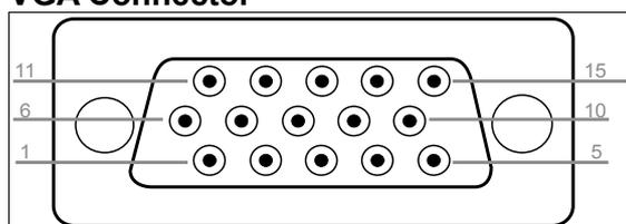
Figure 36: Female VGA Connector HDSUB15 for Carrier Board
