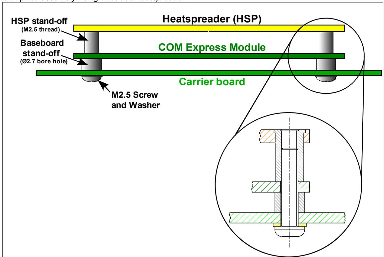
**Note** The torque specification for heatspreader screws is 0.5 Nm.
