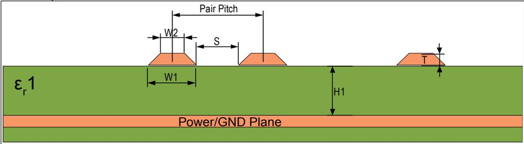
Figure 72: Strip Line Cross Section
