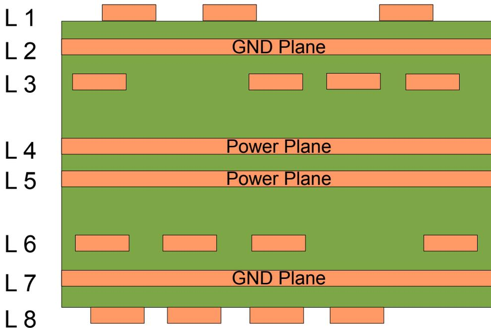
Figure 70 above is an example of an eight layer stack-up. Layers L1, L3, L6 and L8 are used for signal-routing. Layers L2 and L7 are solid ground planes, while L4 and L5 are used for power.
