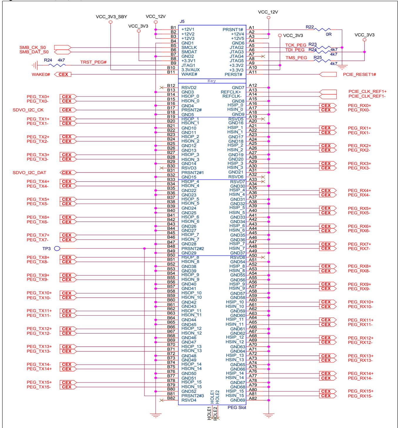
The x16 connector usually is used to drive the PCI Express Graphics Port (PEG) consisting of 16 PEG lanes, which are connected to the appropriate x16 connector pins. For more information about the signal definition of the PEG port, refer to Section 2.4. 'PEG (PCI Express Graphics)' on page 48 above.
