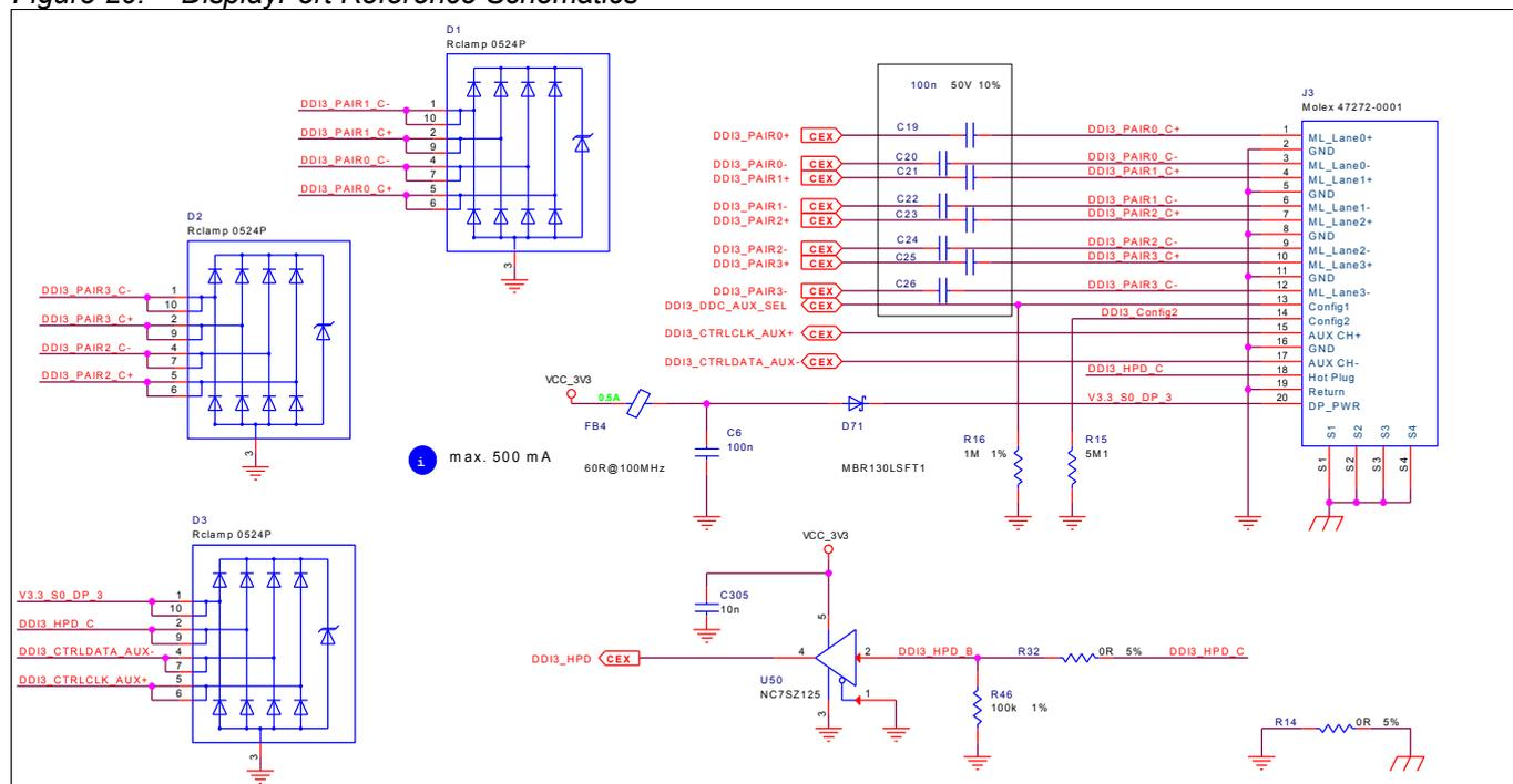
DisplayPort is directly supported by a dual-source DDI. ESD protection, DC blocking capacitors and hot plug detect are the only components required.
