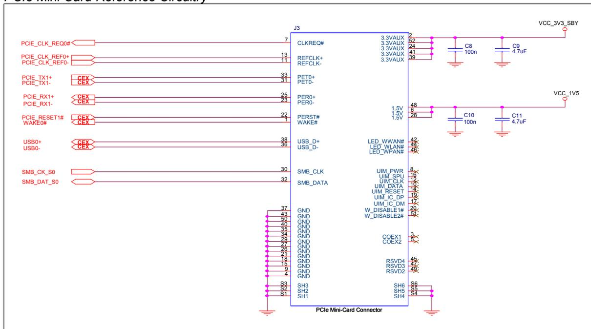
A PCI Express Mini Card schematic example is shown in Figure 14 above. The reference clock pair is sourced from the zero delay clock buffer shown earlier in Figure 6 'PCIe Reference Clock Buffer' on page 35 above. The clock pair is enabled when the PCI Express Mini-Card pulls its CLKREQ# pin low.
