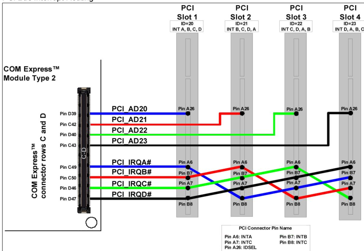
Most of these PCI devices only utilize the interrupt signal 'INTA#'. To distribute the interrupt source of the devices over the interrupt signals 'INTB#', 'INTC#' and 'INTD#', an interrupt cross routing scheme has to be implemented on the COM Express Carrier Board design. Figure 59 above and Table 49 below illustrate the PCI bus interrupt routing for the PCI bus slots 1-4.
