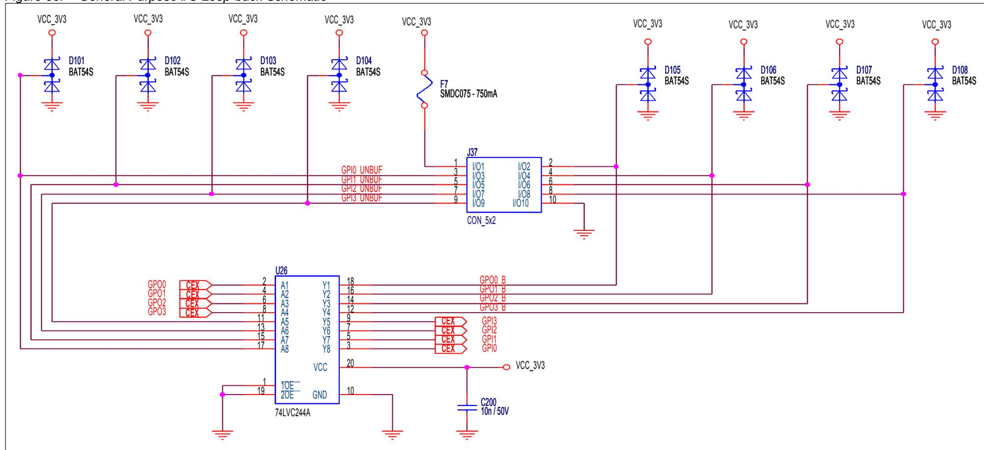
There are 4 GPI (General Purpose Inputs) and 4 GPO (General Purpose Outputs) pins in Figure 55 above.
