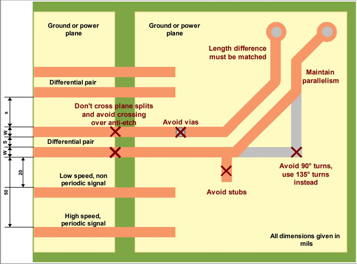
In order to determine the necessary trace width, trace height and spacing needed to fulfill the requirements of the interface specification, it's necessary to use an impedance calculator.
