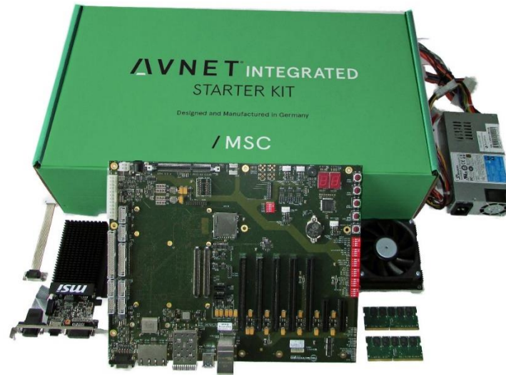
Sample image of a Starter Kit for MSC COM modules (here: COM Express Type 7)
