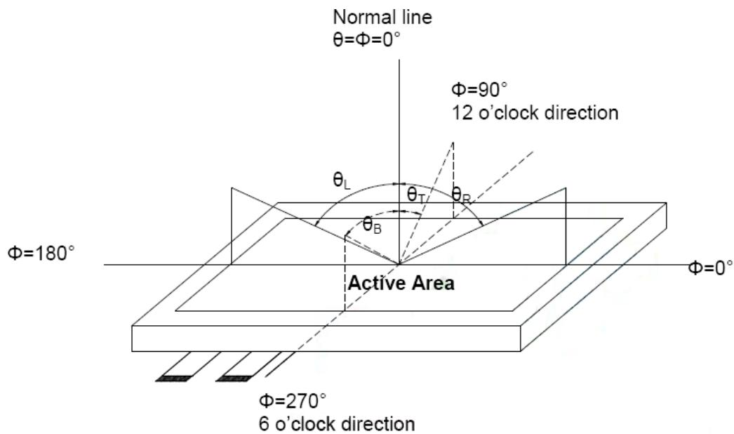
Note (2) Definition of optical measurement system
