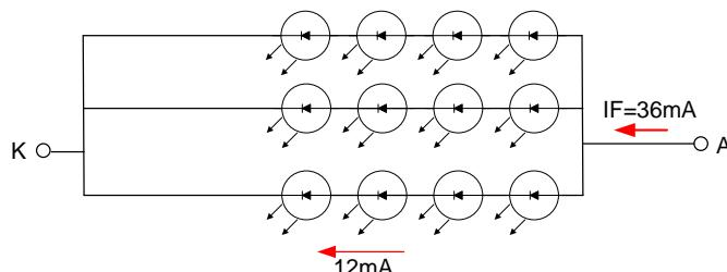
Note 4: When LCM is operated over 60°C ambient temperature, the  $I_F$  of the LED back-light should be adjusted to 18mA max
