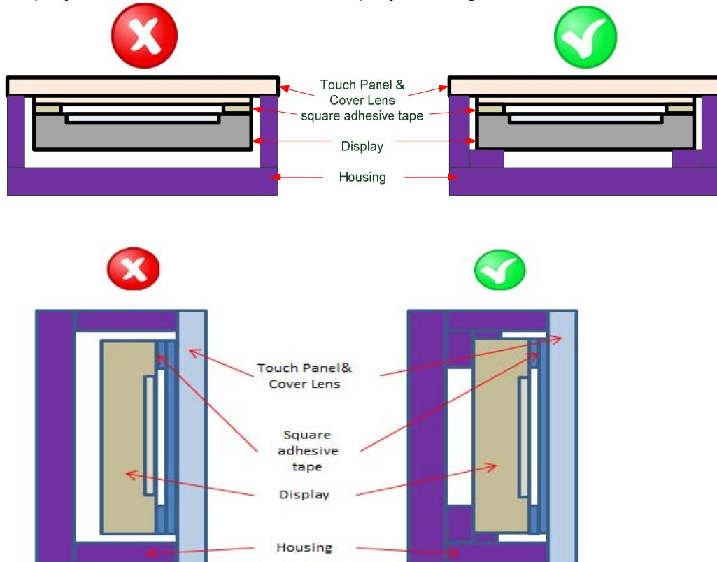
(3) TP needs to work in environment with stable stray capacitance. In order to minimize the variation in stray capacitance, all conductive mechanical parts must not be floating. Intermittent floating any conductive part around the touch sensor may cause significant stray capacitance change and abnormal touch function. It is recommended to keep all conductive parts having same electrical potential as the GND of the touch controller module.
