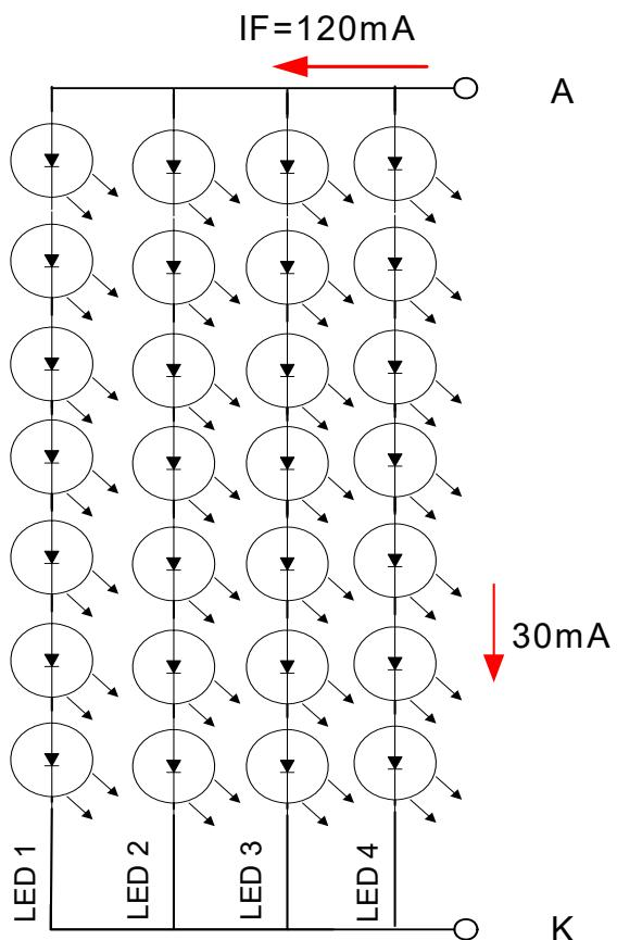
Note(3) When LCM is operated over  $40^{\circ}\text{C}$  ambient temperature, the IF should be follow :
