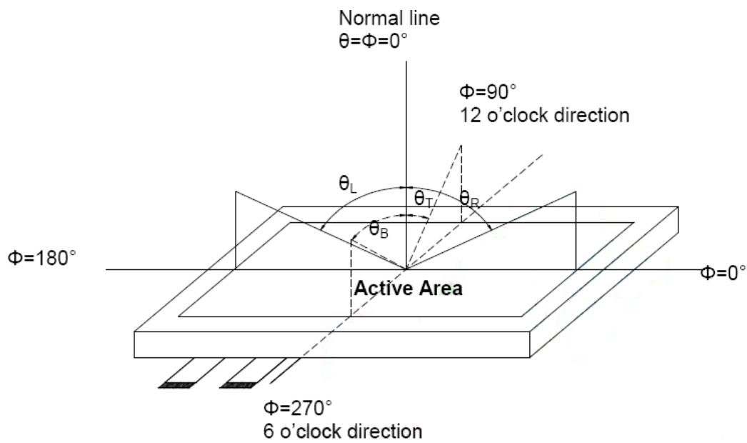
Note (2) Definition of optical measurement system
