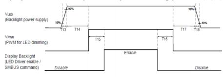
Note: When the adapter is hot plugged, the backlight power supply sequence is shown as below.
