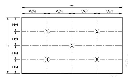
**Note 2**: The luminance uniformity of 5 points is defined by dividing the maximum luminance values by the minimum test point luminance
