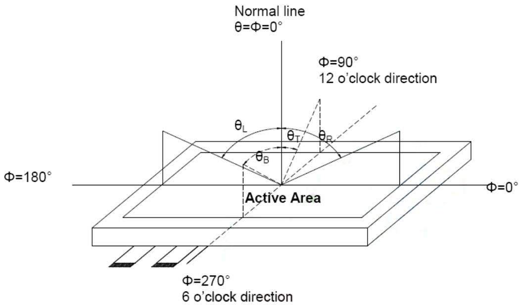
Note (2) Definition of optical measurement system
