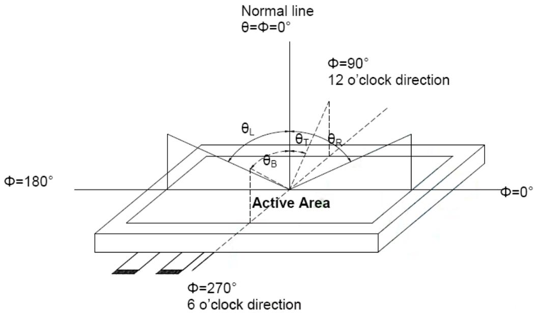
Note (2) Definition of optical measurement system
