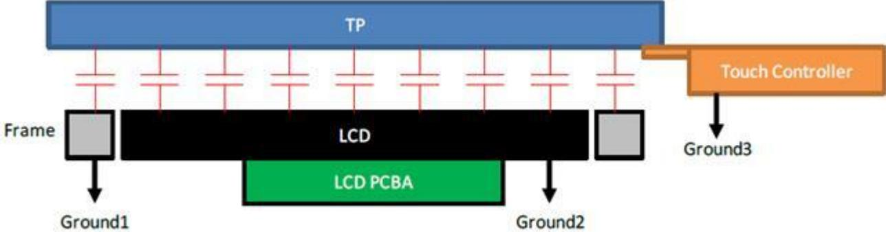
GND1, GND2 and GND3 should be connected together to have the same ground
