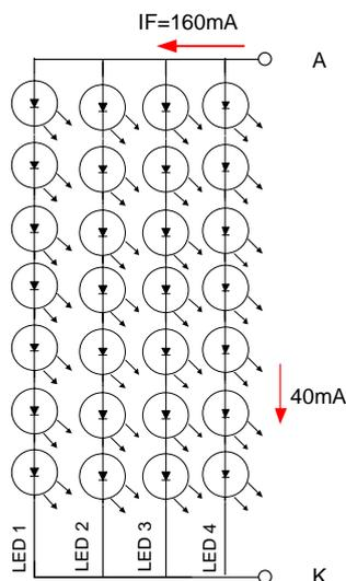
When LCM is operated over 40°C ambient temperature, the IF should be follow :
