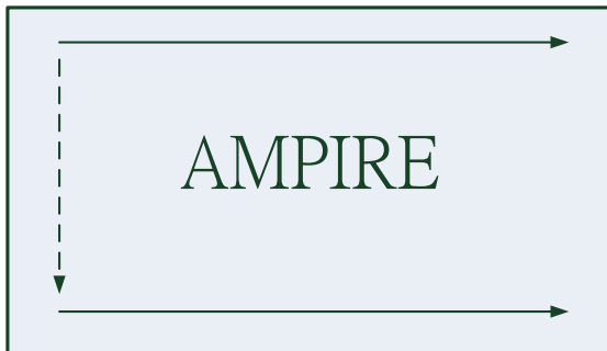
Fig. 1 Normal scan (pin 4, LR/UD = High or NC)
