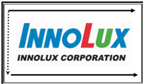
Fig. 1 Normal scan ( pin 4, LR/UD = High or NC )
