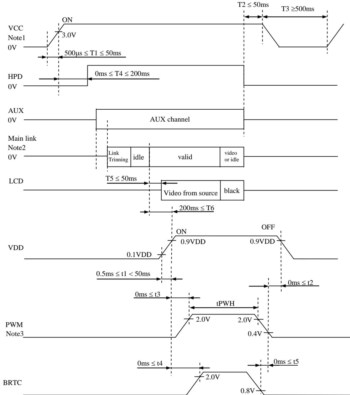
Note1: If there is a voltage variation (voltage drop) at the rising edge of VCC below 3.0V, there is a possibility that a product does not work due to a protection circuit.
