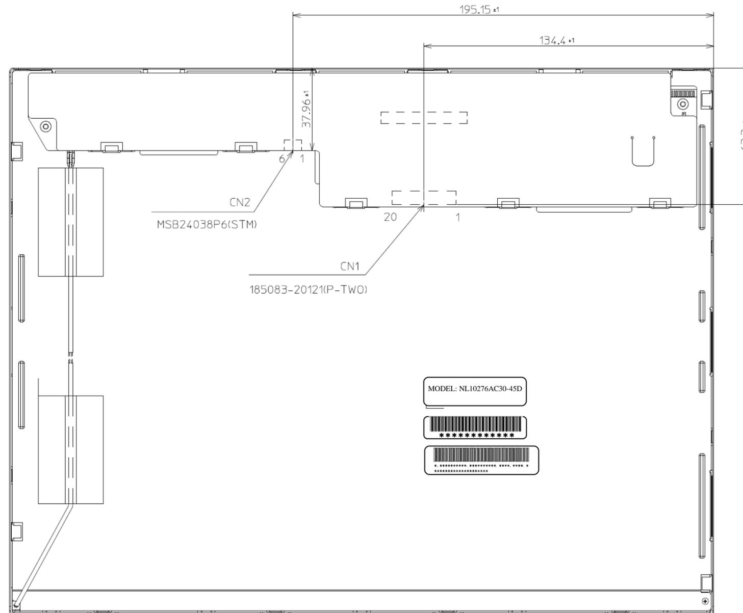
Note1: The torque for product mounting screws must never exceed 0.392N·m. And the length of product mounting screws must be  $\leq 4.5$  mm.
