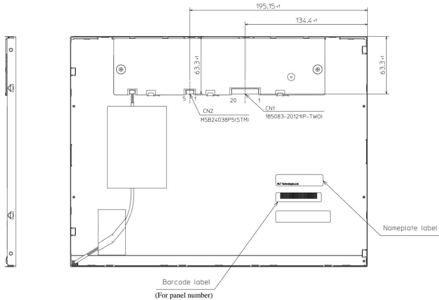
Note1: The torque for product mounting screws must never exceed 0.392N·m. And the length of product mounting screws must be  $\leq 4.5$ mm.
