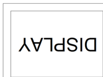
Fig. 9.11 Rotation of 180 degree (U/D: Low; L/R: Low)
