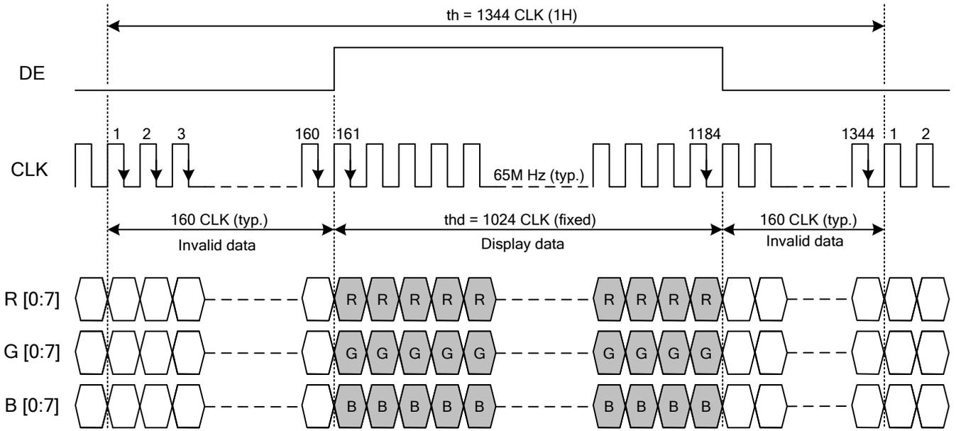
Fig. 9.1 Horizontal Timing
