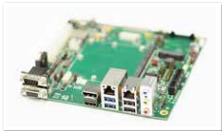
SMARC® Evaluation Platform EP1
